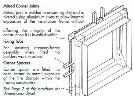
The frame is designed to allow, under fire conditions, expansion of the damper without distorting the surrounding structure.
